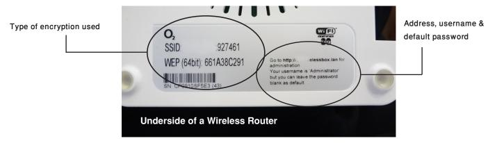
If you set the router password long ago and no longer remember it, you can often reset the password to the manufacturer's default by pressing a reset button or pin on the router itself (holding it down for 20 seconds or so).
